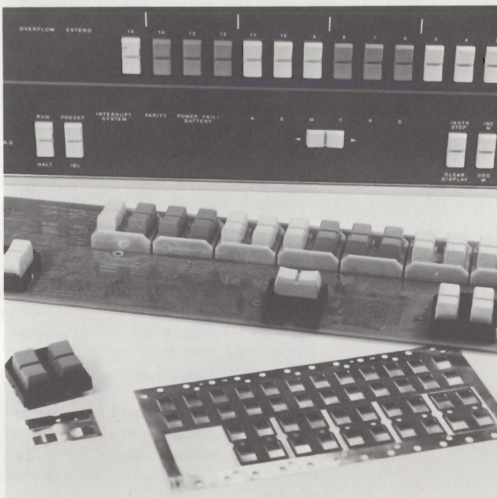
Closeup of keyboard elements shows relationship to keyboard of the HP-35 calculator.
